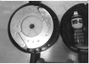
**NOTE:** Make sure that the reel and electric tape stays in place in the bottom half, as in the picture above. And put the plastic washers that is fitted between the center shaft and halves back in place before reassembling.
